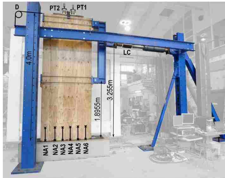
Figure 2.9: Test set up as reported by (Sarti et al. 2016).
